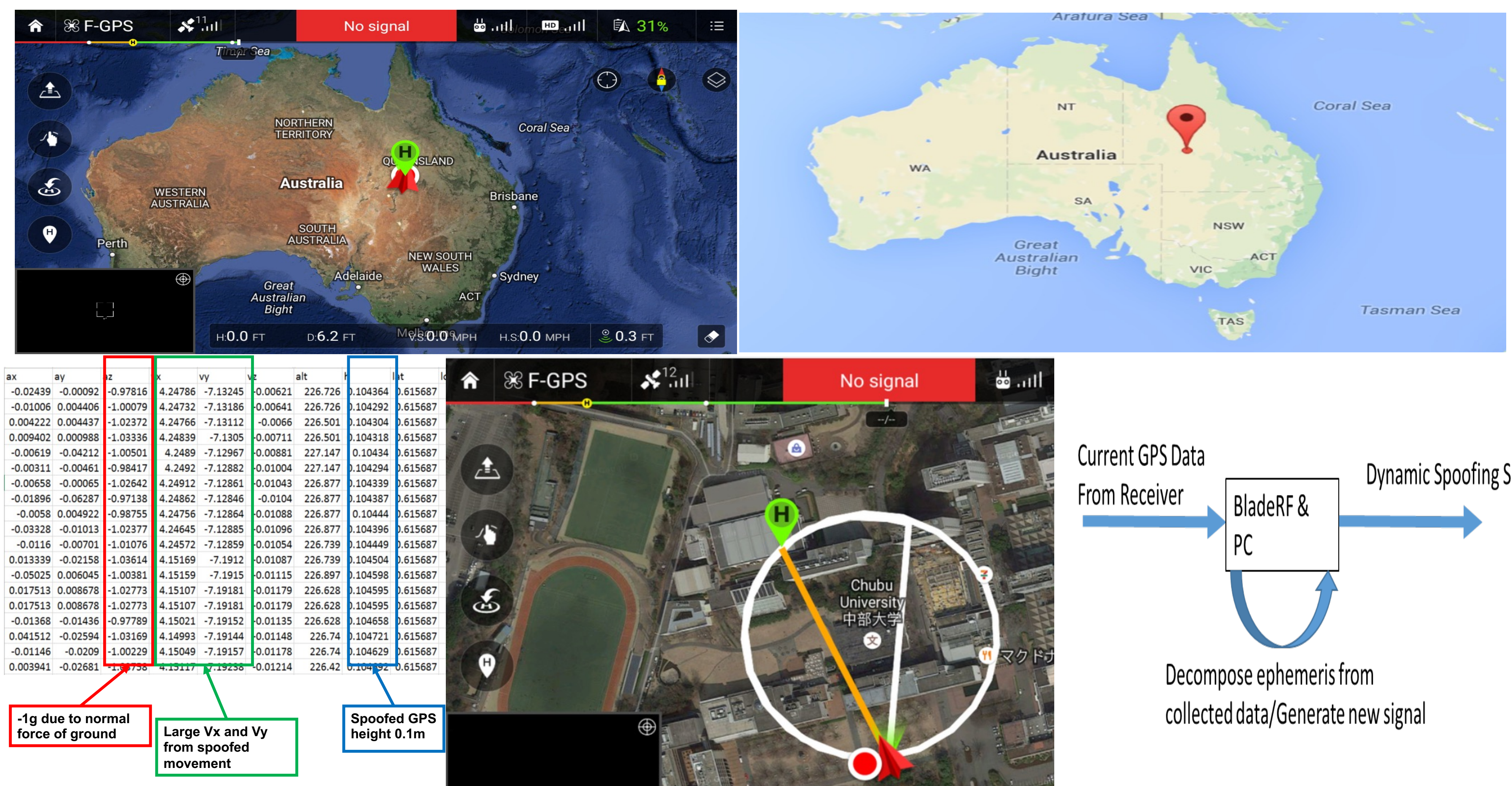
Figure 3: Dynamic Spoofing Signal Generation
