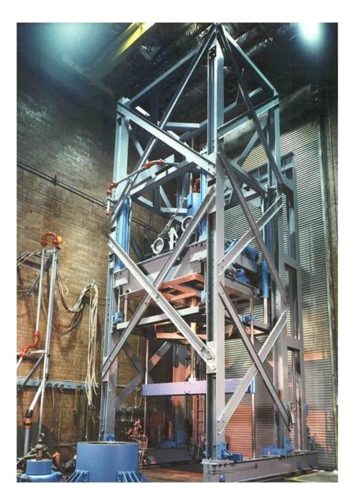
Large Sample Pressure Sealing for Pressure Drilling Tests 1978
